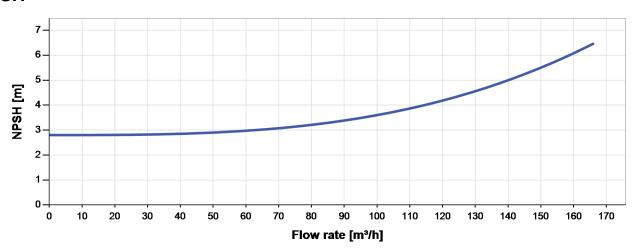
The NPSH (Net Positive Suction Head) is NOT the operating suction head. To calculate the operating suction head please refer to the installation manual.
